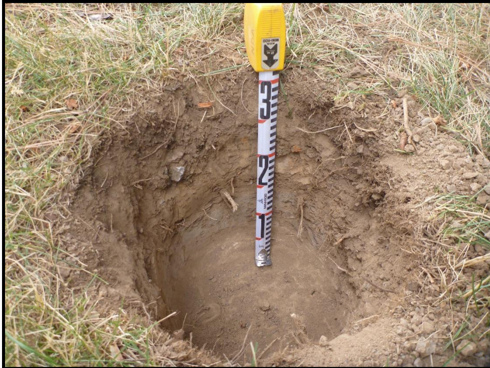
Image 17: Test Pit – Disturbed
