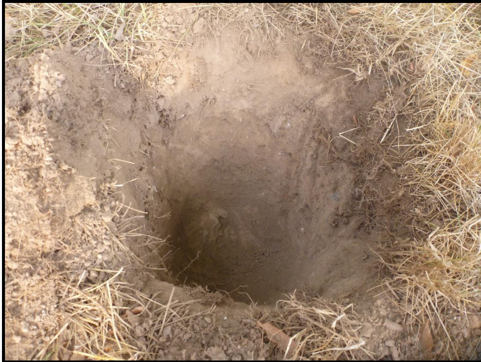
Image 15: Test Pit – Disturbed
