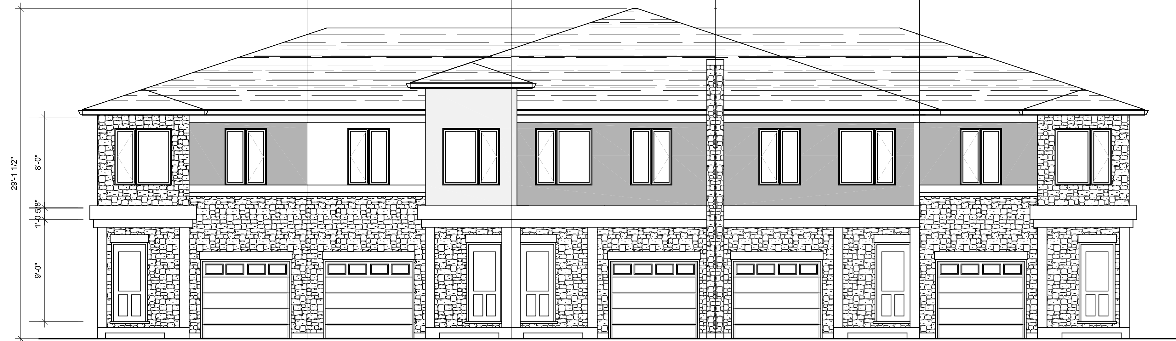
1 FRONT ELEVATION BLDG D TYPE B REV END TYPE B TYPE C TYPE C REV TYPE B END A103 3/16"=1'-0"
