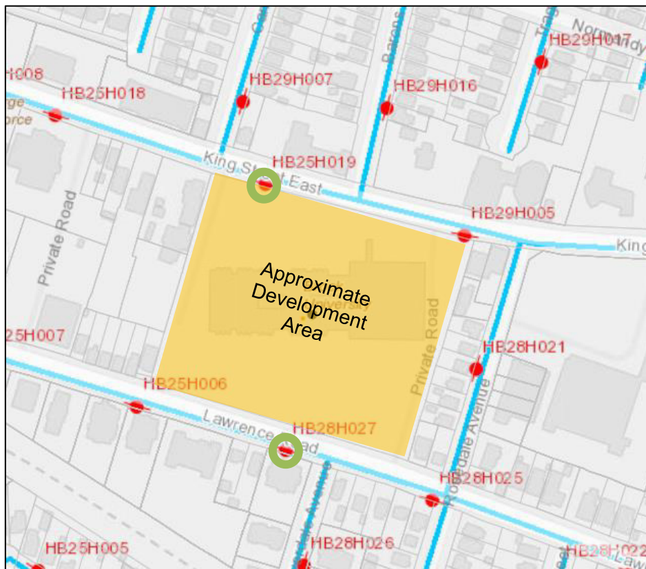
Figure 3-1: Hydrants used for Model Validation
