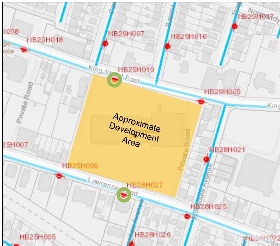
Figure 3-1: Hydrants used for Model Validation
