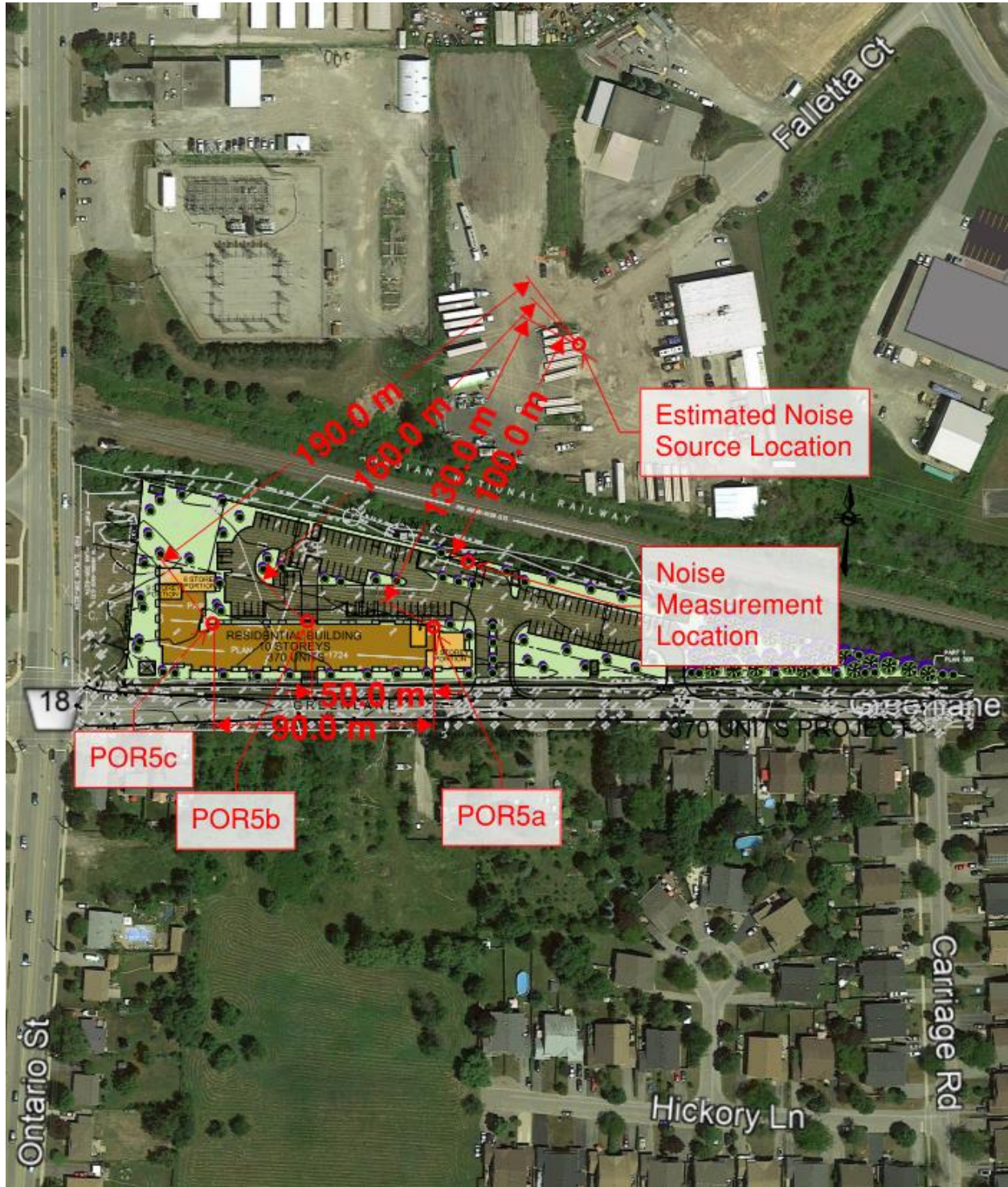
Figure 1: Noise measurement and point of reception (POR) locations (Level 8 of the north façade)
