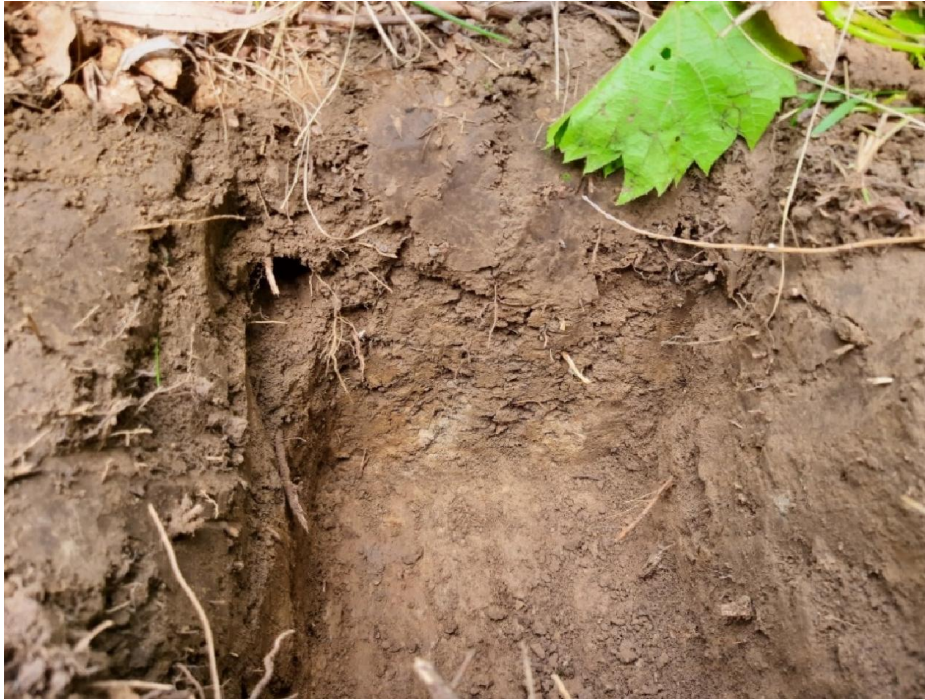
Image 11: Typical disturbed soil profile in south and central portions; transition between fill and sterile B-horizon not easily distinguished on visual basis.
