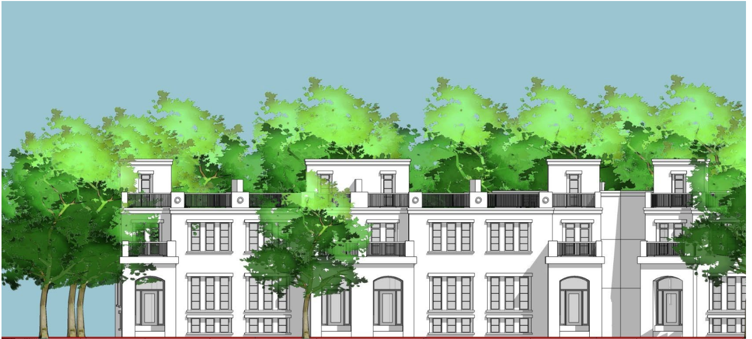
Scenic Dr. massing concept showing a 2 storey wall height with roof terrace access extended into the 3 rd floor. Note principal entrance.
