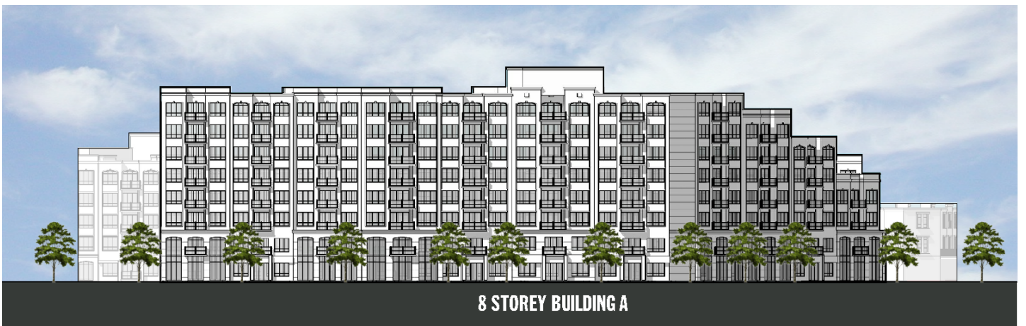
Building A proposed at 8 storeys with a 2 storey base. Upper floors are stepped back toward the Brow edge to reduce visual presence. Building plan is cranked to further diminished the perceived mass. (KNYMH Architects)
