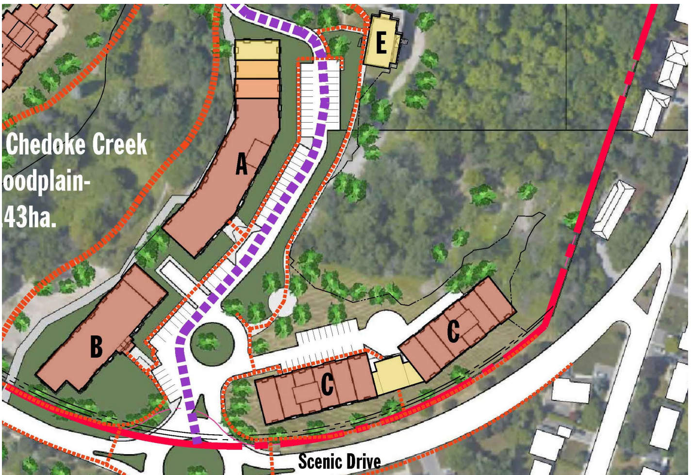
Block 2 Precinct Plan with mid-rise buildings organized along a north-south driveway
