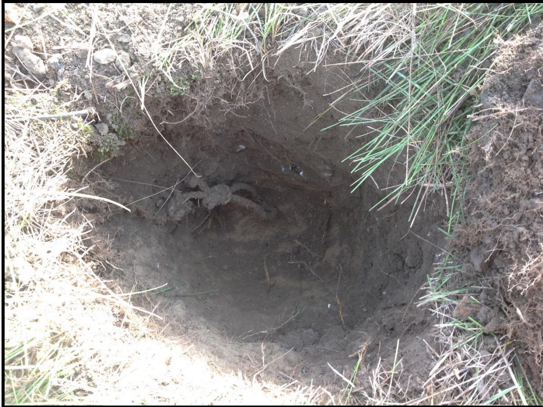
Image 7: Example of a disturbed test pit, note rope, asphalt inclusions
