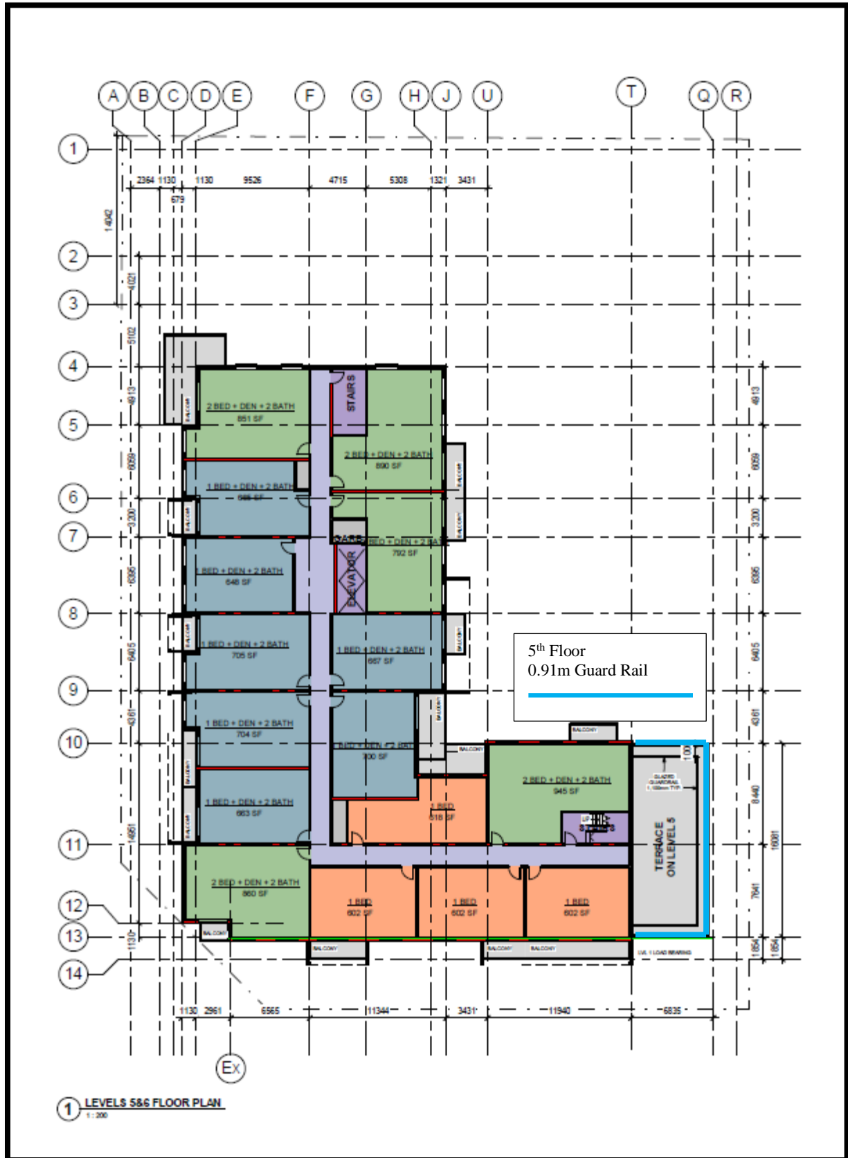
FIGURE 3 5 th FLOOR 0.91m GUARD RAIL
