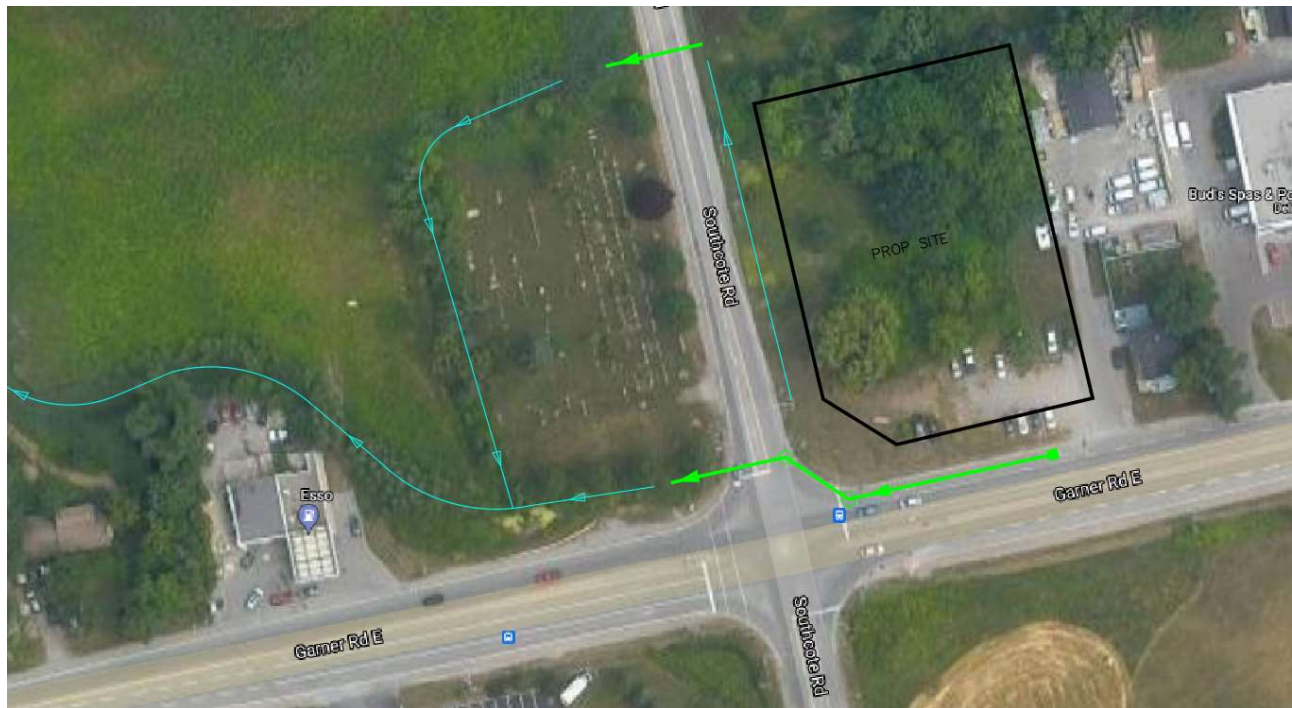
Figure 2 – Existing Storm Drainage Pattern
