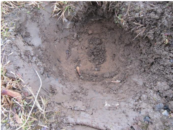
Photo 33: Sample test pit #6 with buried aggregate layer, potential septic field
