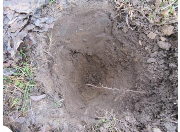
Photo 32: Sample test pit #5 revealing stone pad
