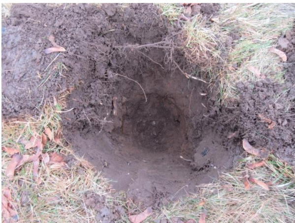
Photo 33: Sample test pit #6 with buried aggregate layer, potential septic field
