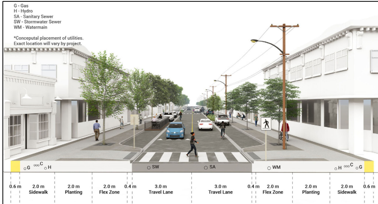
Figure 25 – 20 m ROW Main Street Typical Cross-Section Design
