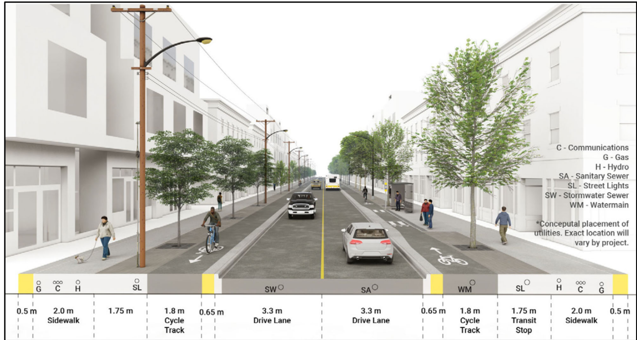
Figure 23 – 20 m ROW Urban Avenue Typical Cross-Section Design
